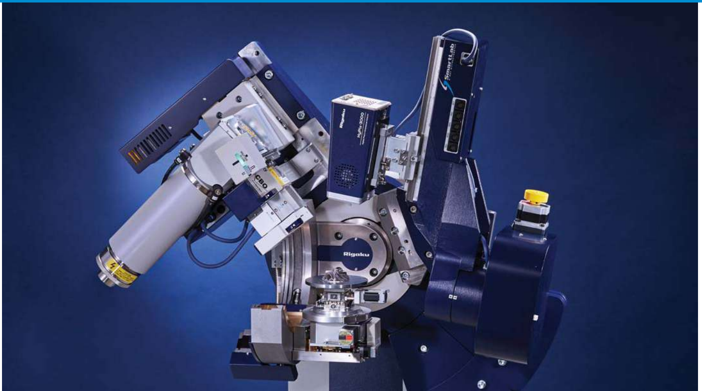
Residual Stress measurement optical configuration
